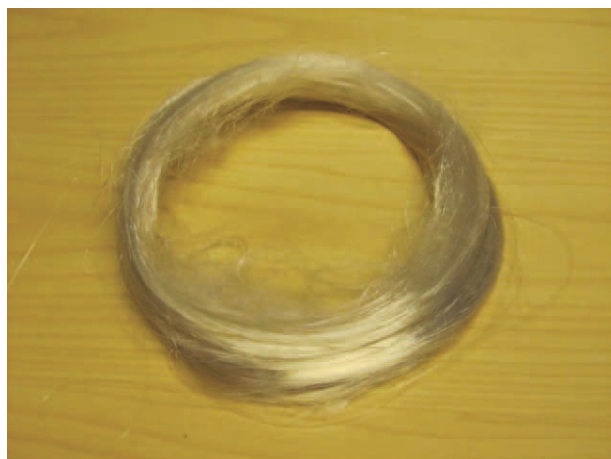
Figure 6 Spun PEEK filaments. [Color figure can be viewed in the online issue, which is available at wileyonlinelibrary.com .]
